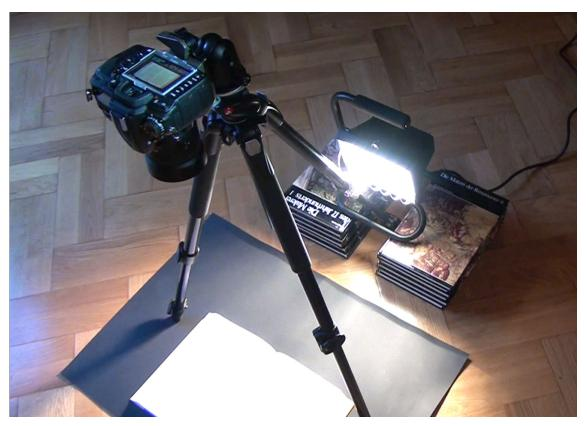
Figure 3.1 Hardware setup for scanning.
